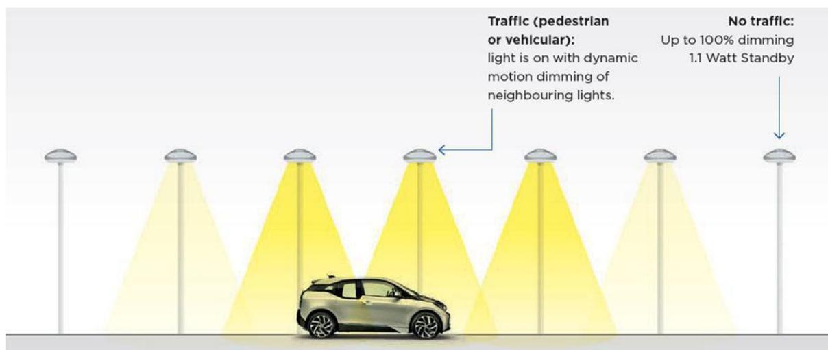
Compared to normal LED street lighting you increase energy efficiency up to 90% with the intelligent lighting system. This extends the lifetime of the luminaires and reduces maintenance costs.
