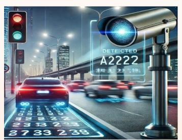
Automatic Number Plate Recognition (ANPR) is a technology used to automatically read the license plates of vehicles. It is commonly employed in various applications such as traffic monitoring, law enforcement, parking management, toll and collection. systems ANPR capture images of vehicles using high-definition cameras, which are then processed to detect the vehicle's license plate. The first step in **ANPR** image
